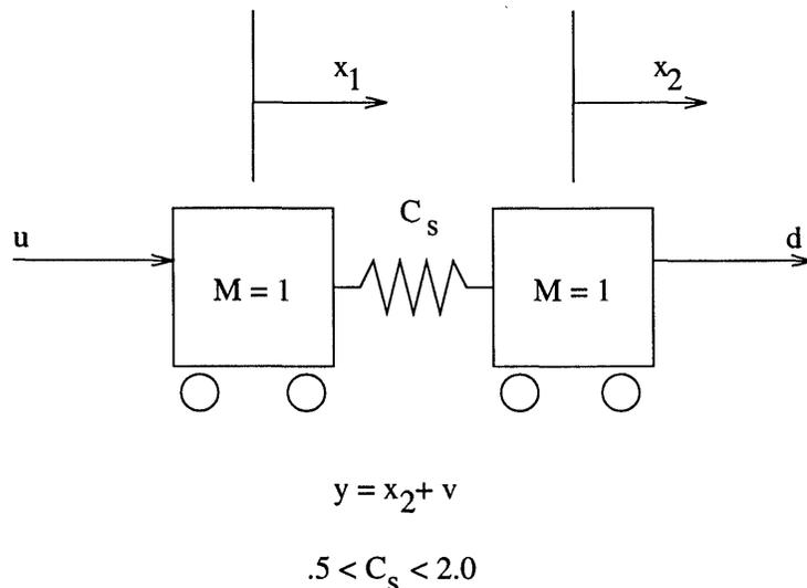
Figure 2: Schematic for the mass-spring system.
