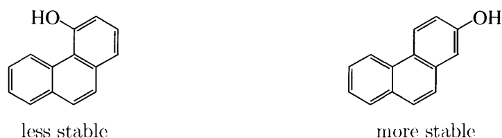
Figure 4-5: Benson’s method does not differentiate the groups according to where in the PAH the substituent is located, although it is known, for example, that a substituent at a bay region leads to a higher energy than a substituent in another position, due to steric interactions.
