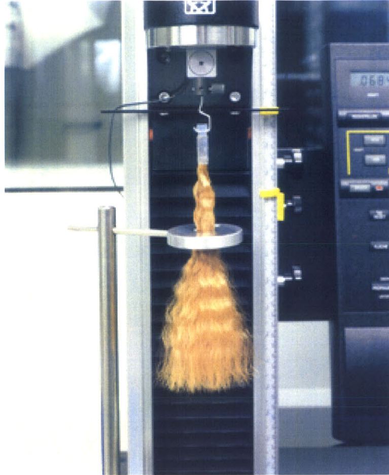
Figure 2-16: Volume measurement test setup at Wella FKM Laboratory in Darmstadt, Germany [ right ], and image acquired by the system with image analysis of style volume applied [ left ]. (Taken from archives, Wella AG)
