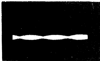
Fig. 3-13 Signal Modifier (With Filters) Output for w_c = 377 Rads/sec and w_d = 6.35 Rads./sec.
