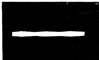
Fig. 3-14 Signal Modifier (With Filters) Output for w_c = 383.3 Rads./sec and w_d = 6.35 Rads./sec.
