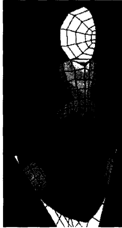
(a) The shell model with a modulus of 0.1 kPa for the PCM fit the experimental data well for day 28 FBS cultured cells. Note that the color scale of (a) and (b) are not the same.
