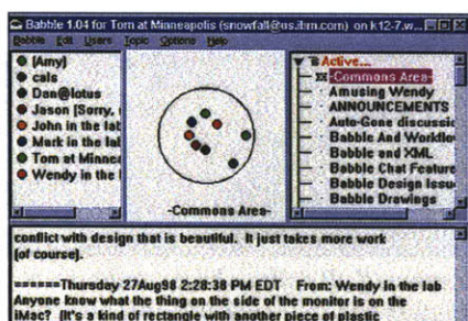
Figure 16: The Babble system from IBM. The top middle panel shows all logged in users, with more active ones being drawn to the center of the circle.
