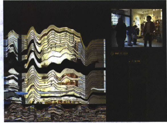
Figure 40: History Display showing the growing stack of layers on the left. Within the stack, the currently selected layer is highlighted with yellow lines outlining it. To the right we see the image from the currently selected layer from the stack. Below the image we see indication of the day and time this image was captured.
