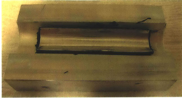
Figure 6-9: Mould semi-cylindrical cavity with oversized rubber-metal laminate and cured adhesive.
