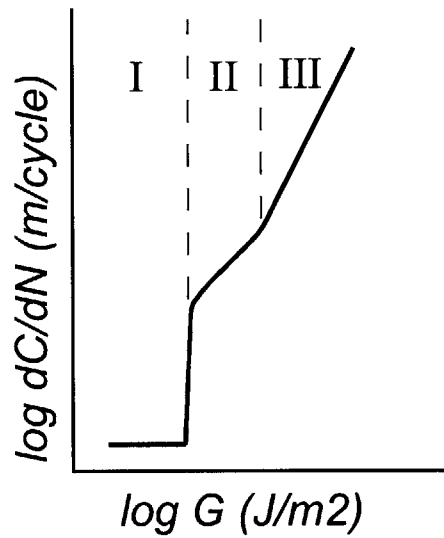
Figure 2-21: Cyclic crack growth rate dC/dN ; data of unfilled Natural Rubber adapted from [9].
