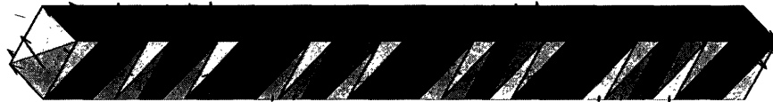
(e) Long thin wire. Over the frequency range, the wire has length .3\lambda to 3\lambda .
