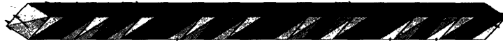
(a) Long thin wire: Over the frequency range, the wire has length .3\lambda to 3\lambda .
