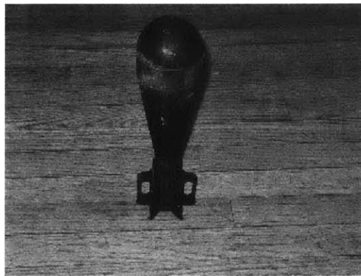
Figure 5-28: An example of UXO with the longest dimension 280mm and widest dimension 83mm, designated U1 (Courtesy of Dr. K. O’Neill)
