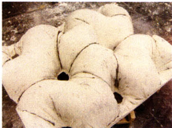
Cast piece is flipped and used as the formwork for the next cast
