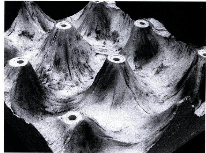
Fig. 101. Full Size Mockup Using Concrete. 2' x 3' segment of a wall.
