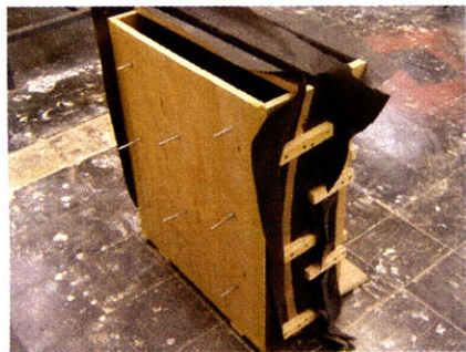
Fabric is hung vertically using steel rods and spacers. Four layers of fabric used to create three panels.
