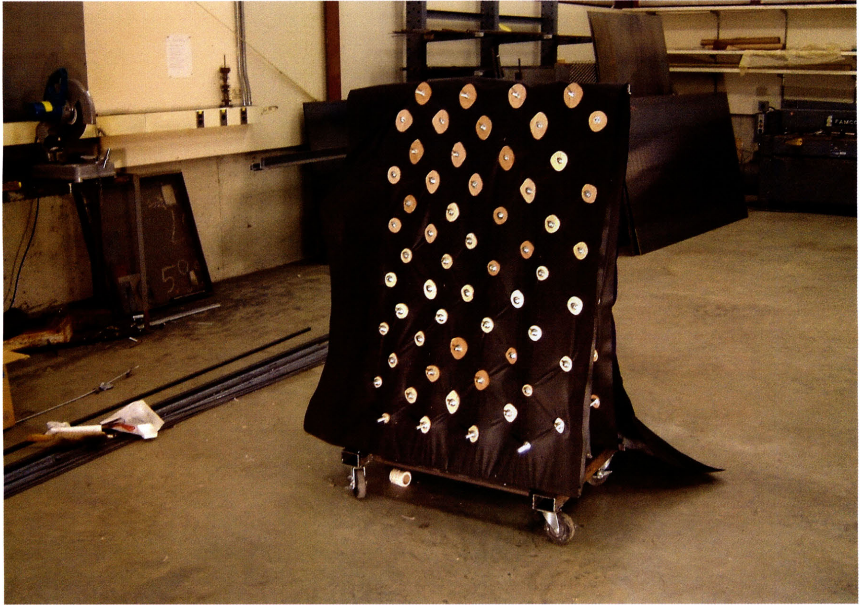
Fig. 164. CONSTRUCTION SEQUENCE 12. The outer fabrics are brought together at top of the frame.
