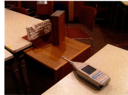
Fig. 146. TEST-ING METHOD. Wall is placed in front of the speaker and the recorder behind the speaker.
