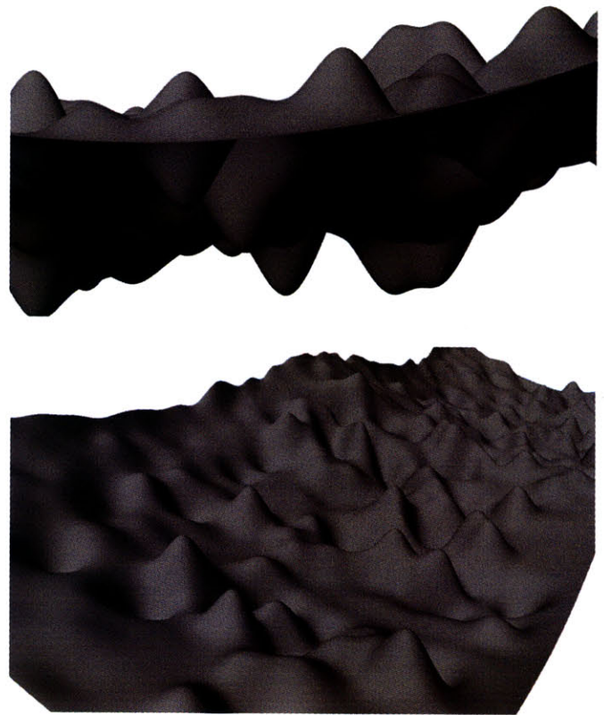
Fig. 119. RENDERINGS OF FABRIC FORMWORK. Show the undulation of the fabric based on the size of spacers. Spacers not expressed in this rendering.
