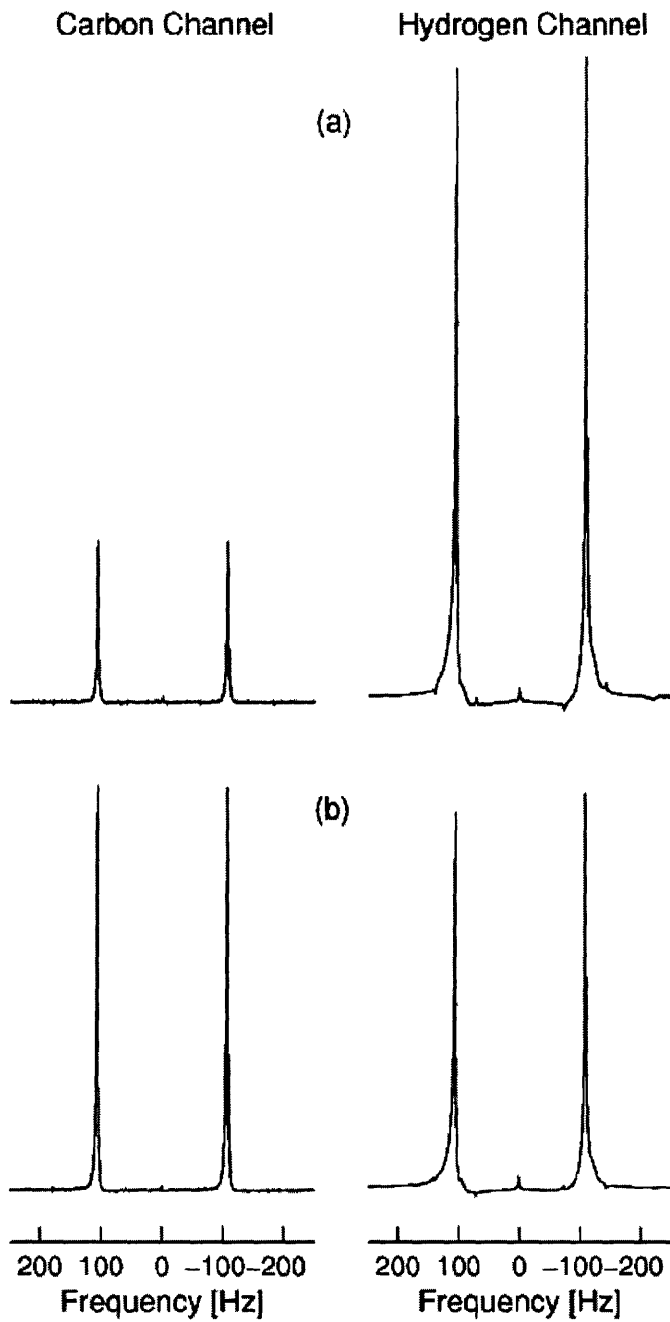
Figure 3-4: Equalizing magnetization Since the ratio of \gamma_H to \gamma_C is a factor of four, the spectra of H and C following a \frac{\pi}{2} pulse should reflect 4 : 1 ratio in the peak heights, shown in (a). In order to compensate the different magnetization, the equalization pulse sequence is applied and results in the spectrum (b).
