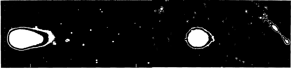
Figure 3-13. A common problem encountered in the comet assay analysis was unclean background. The LACAAS could not handle this situation therefore the results were unreliable. The problem usually came from careless handling of the sample slides so that dirt fell onto the slides and was stained by the fluorescent dye. Data corresponding to these images should be removed from the Excel files before further statistical analysis.
