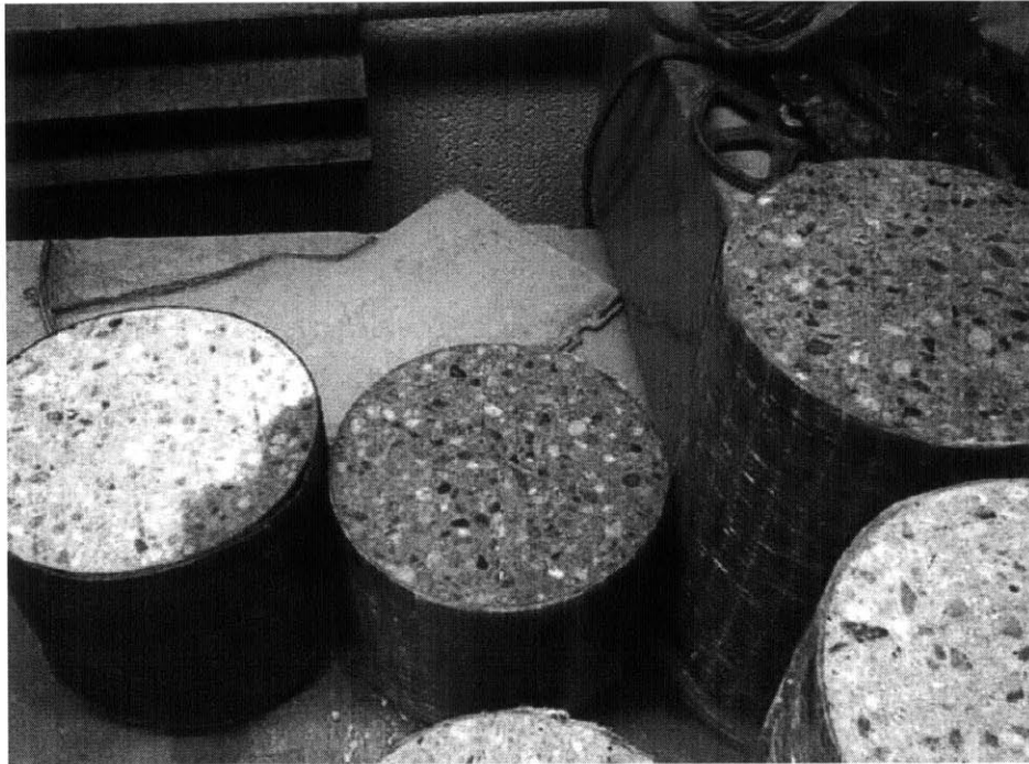
Figure 3-28 Examples of specimens after cutting procedure
