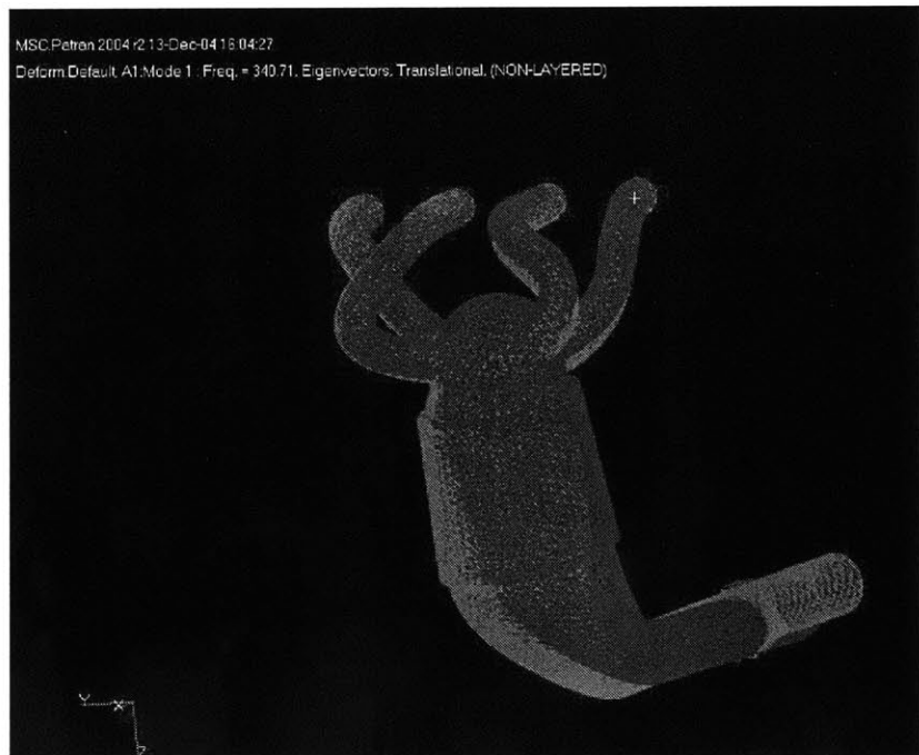
Fig. 84: Modal Shape Visualization (global lateral mode)
