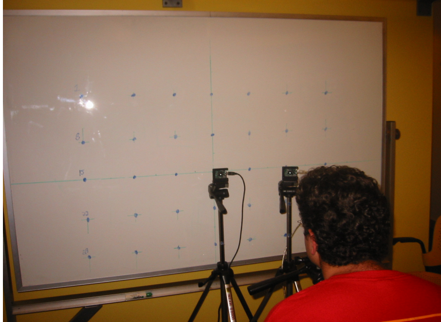
Figure 3-7: Experimental setup used to acquire eye images from 16 subjects with ground truth eye gaze. This dataset was used to train our eye detector and our gaze estimator.
