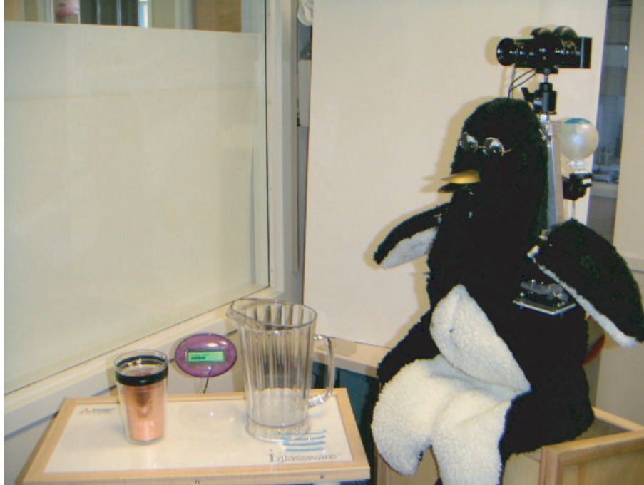
Figure 2-2: Mel, an interactive robot, can present the iGlassware demo (table and copper cup on its right) or talk about its own dialogue and sensorimotor abilities.
