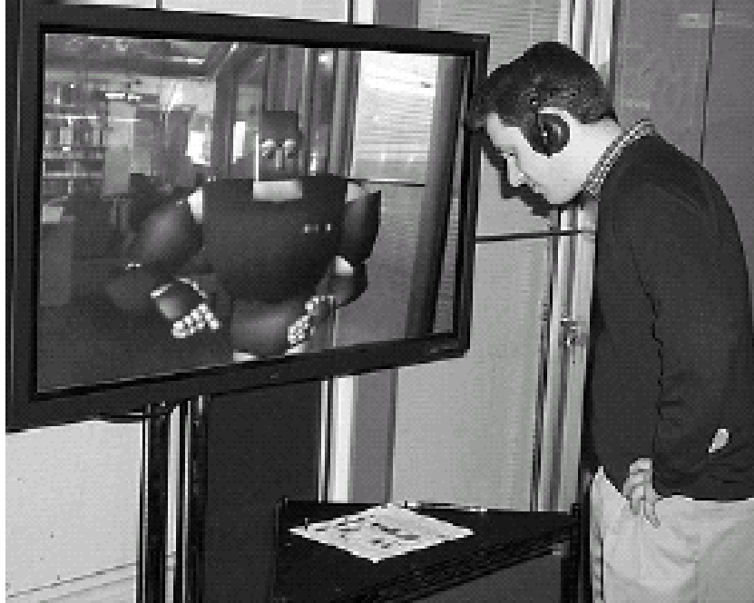
Figure 2-1: MACK was designed to study face-to-face grounding [69]. Directions are given by the avatar using a common map placed on the table which is highlighted using an over-head projector. The head pose tracker is used to determine if the subject is looking at the common map.
