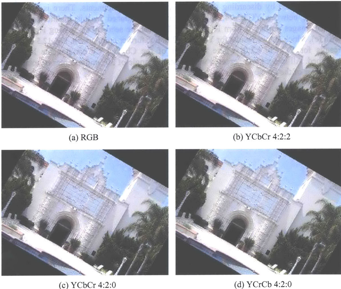
Fig. 12.5. Comparison of rotated images for 4 different color formats. Angle of rotation is 30° clockwise.
