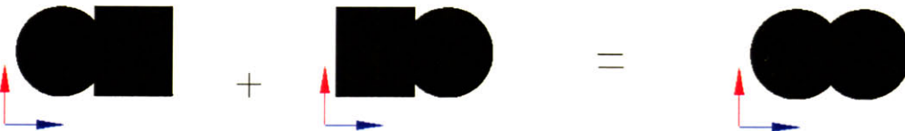
Figure 3-3. Diagram showing pattern combination of two disk patterns, a) shows the commonly expected resulting pattern that is incorrect, b) shows the actual pattern resulting from the combination of the two disks, c) shows what patterns need to be combined to form the desired pattern of a).
