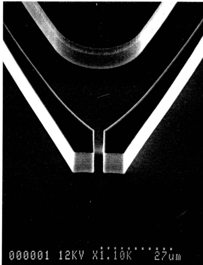
Figure 3-10. SEM photo of structure formed by the FARDAD DRIE process showing the smooth side walls created by the process.
