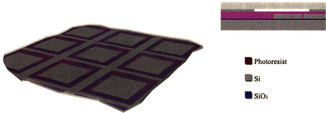
Figure 3-15. Process flow diagram showing the device wafer mounted to a mount wafer a). The mount wafer has special pillars and channels surface micromachined into its interface surface with the device wafer. The locations of these pillars and channels relative to the device wafers are shown in a see through diagram b).
