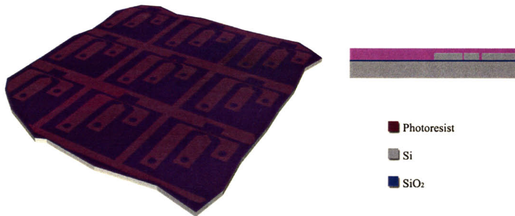
Figure 3-14. Process flow diagram for nanotweezers structures at the completion of step 4 (post PR brace). Insert on the right shows a perspective view of a representative 3 \times 3 die section of the wafer.
