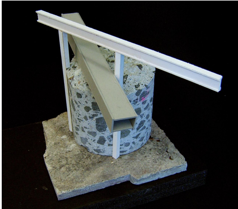
Sketch model of bundled box-beam and columns (white) going down to bedrock and negotiating around tunnels (gray)
