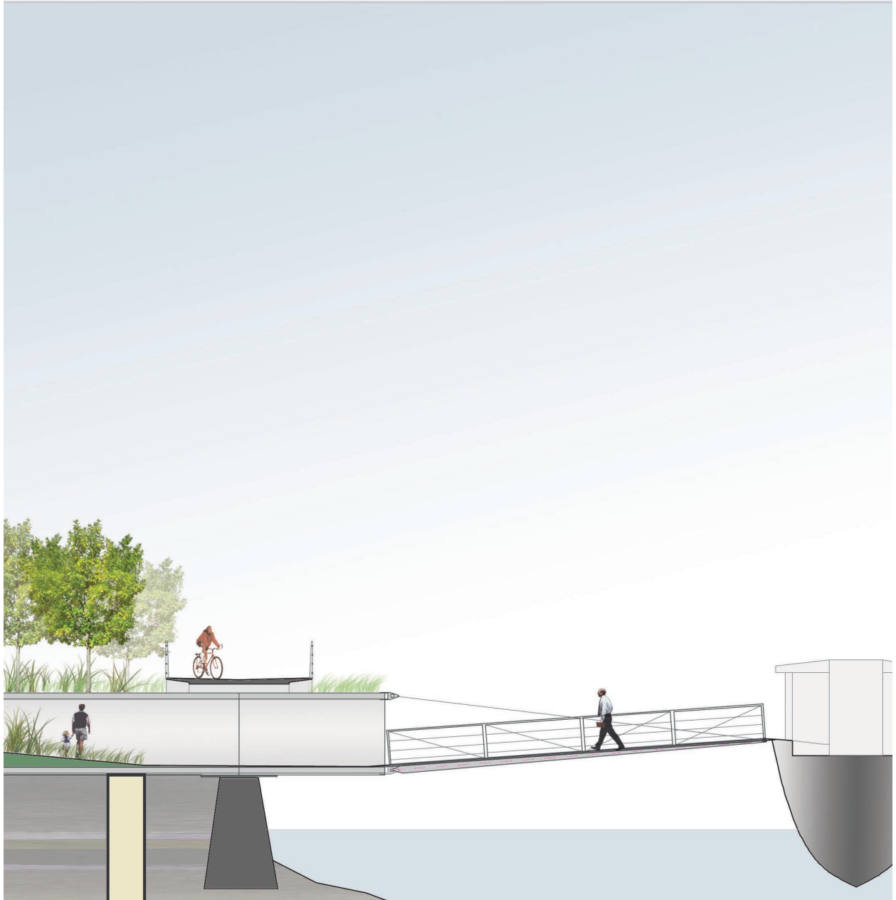
Pier section with shoreline bicycle path occurring overhead and adjustable tension cable for platform leading to watercraft
