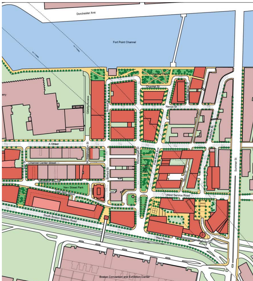
Plan for new buildings (red) and park areas added to existing structures (purple) without regard for tunnels beneath (diagonal lines) [BRA 2005]
