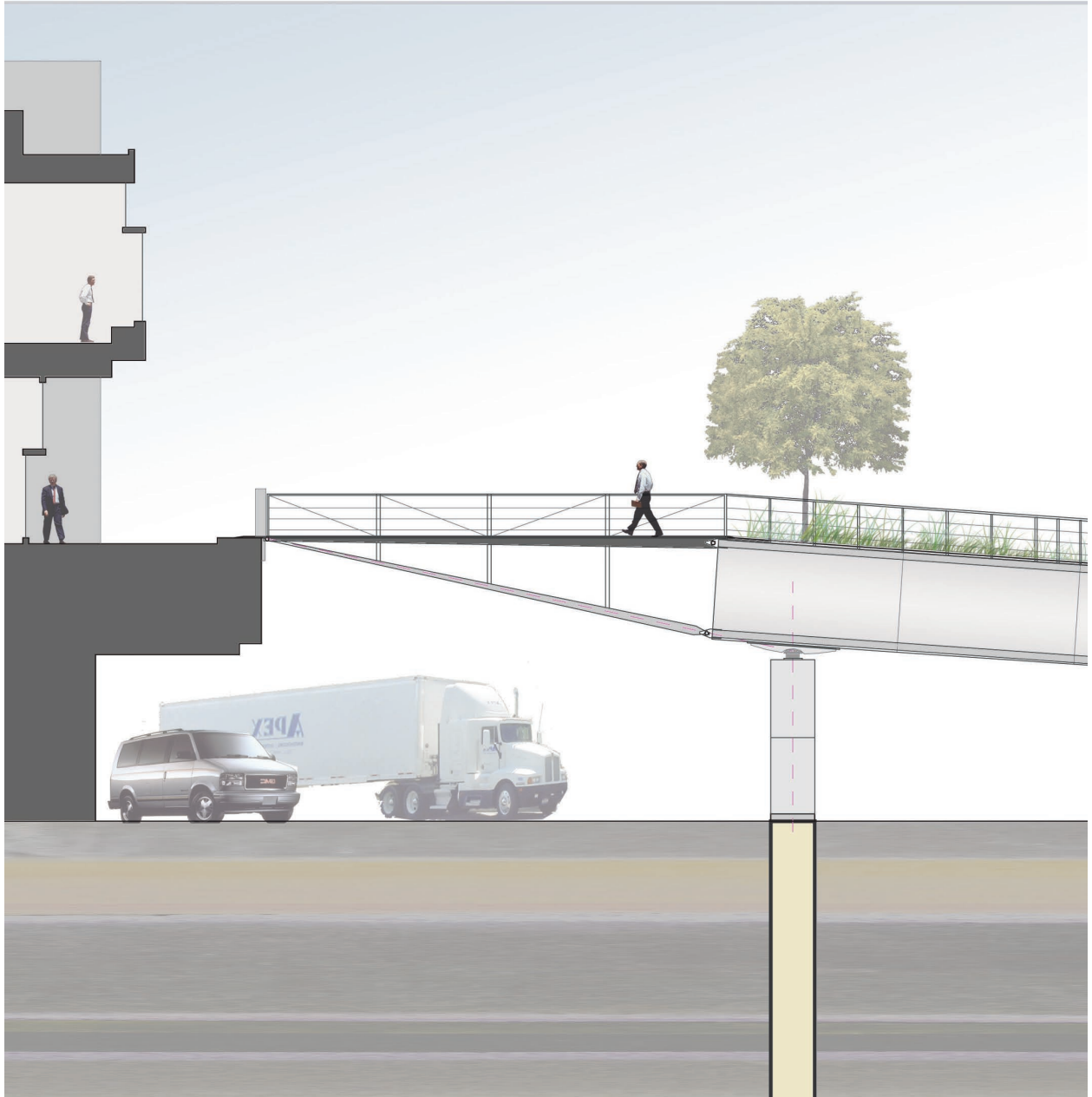
Section through convention and loading dock levels and connection to bundles with plantings and pathways
