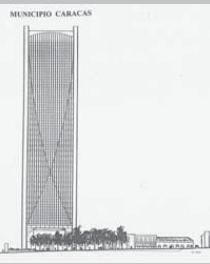
↑ Paired funicular braces create a graceful symmetry of curves.
