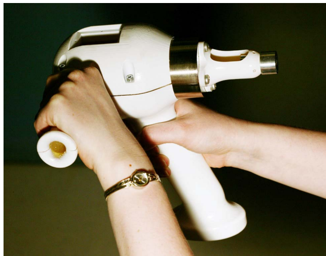
Figure 17: Rapid-prototype of conceptual design of a handheld controllable needle-free injector.
