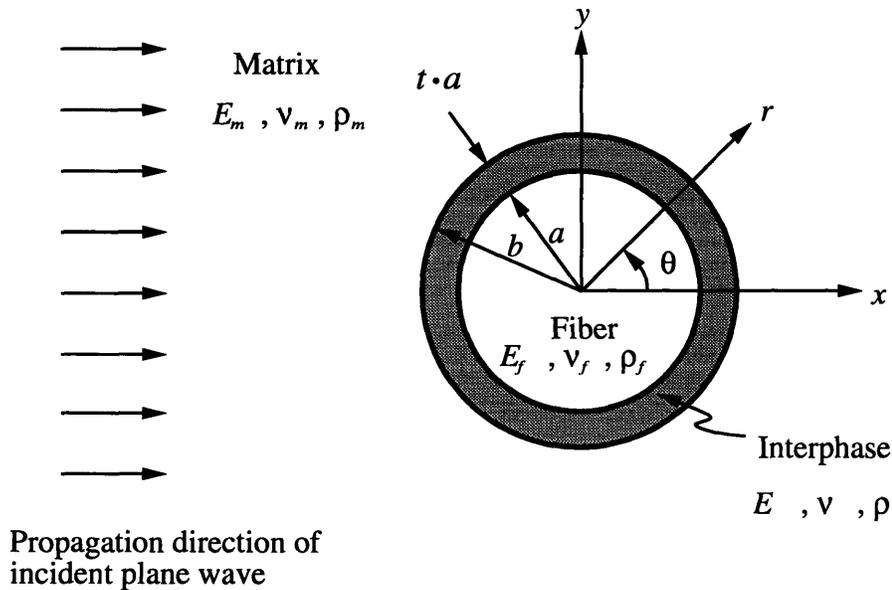
Figure 2-1: Two-dimensional model of single fiber scatterer.
