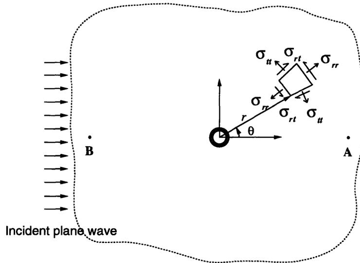
Figure A-3: Wavefield stress components.
