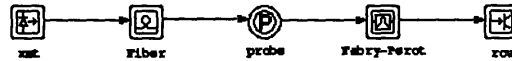
Figure 5-12: Node level description of network for testing the Fabry-Perot filter. The pulse entering the filter is the same pulse generated in section 5.1.2, a gaussian chirped by SPM.
