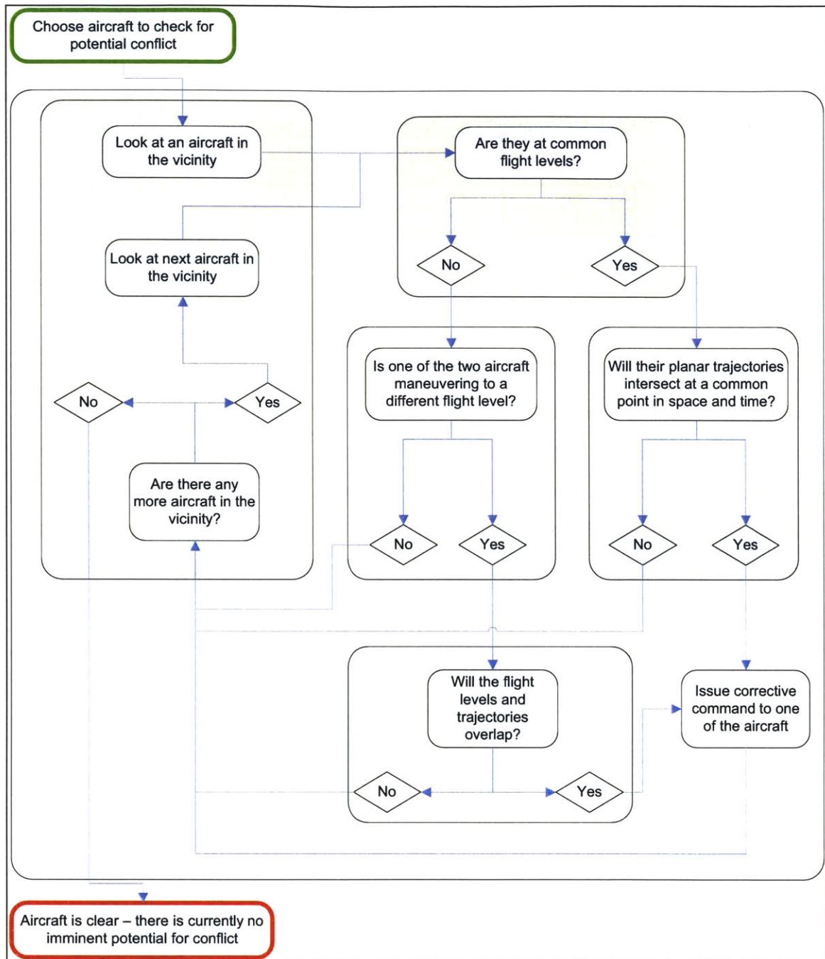
Figure 3-14. Cognitive process of conflict detection for a given aircraft relative to nearby aircraft
