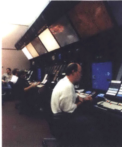
Figure 1-1. Air traffic control human-machine interface. The station shown is the Display System Replacement (DSR) used for en-route traffic operations in the USA. Photo courtesy of Federal Aviation Administration (FAA).
