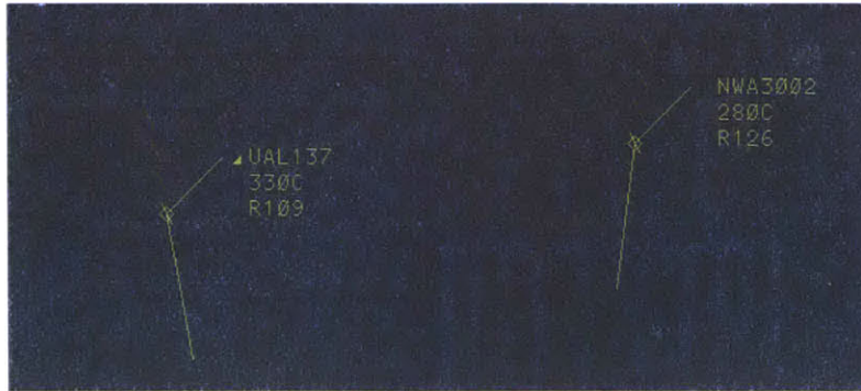
Figure 3-2. Typical en-route ATC display data-blocks showing two aircraft. Data-blocks have three lines of information. The first line of text represents the flight number, the second is the altitude and the third is the computer identification number. Image courtesy of the FAA.
