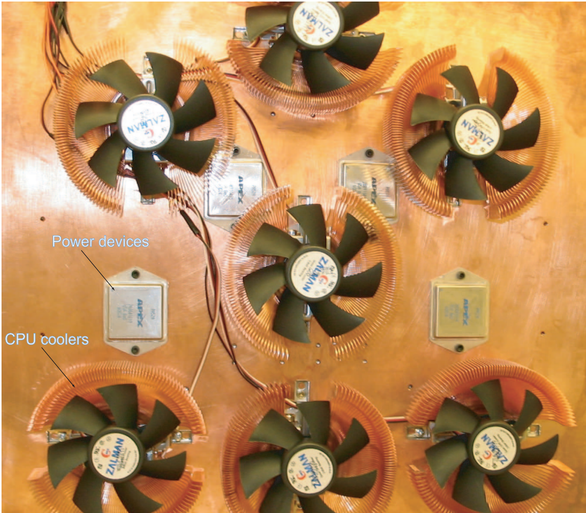
Figure 5-5: The heat sink of the power amplifier
