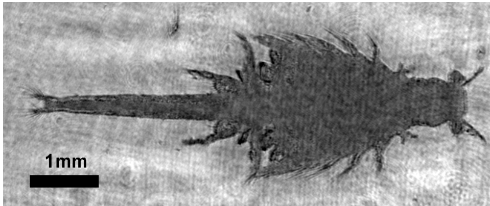
Figure 4-26: Reconstruction of a brine shrimp located 444mm from the CCD.
