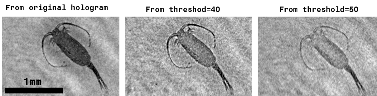
Figure 5-8: Comparison between the original copepod hologram reconstruction and the reconstructions from the two binary holograms at d=114.4\text{mm} .
