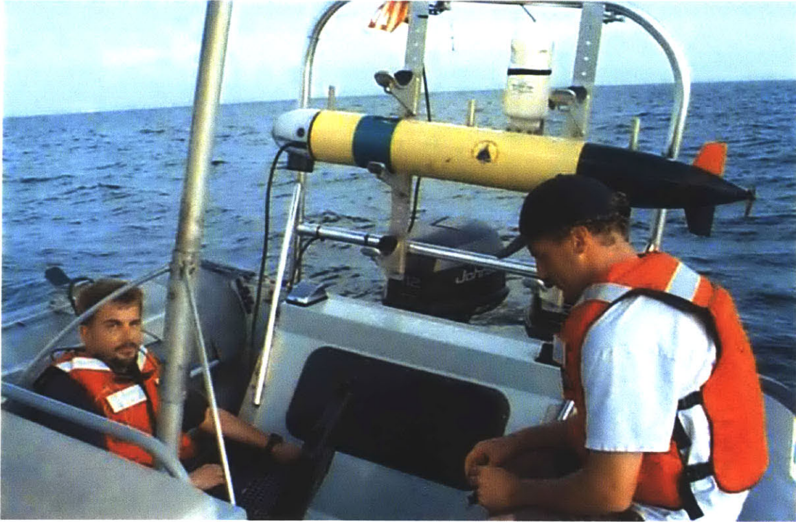
Figure 1-1: The REMUS AUV, developed by the Ocean Systems Laboratory of the Woods Hole Oceanographic Institution (Courtesy of Timothy Prestero).
