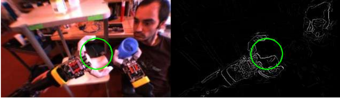
Figure 9-16: Left: The robot’s view during execution of PalmServo . This occurs in an everyday environment which includes a shelf, a person, as well as natural lighting and a cluttered background. The green circles mark the convex shape of the open hand, detected by InterestRegions . This detection is then controlled using TipServo . Right: The motion edges used in the detection of the palm by InterestRegions .
