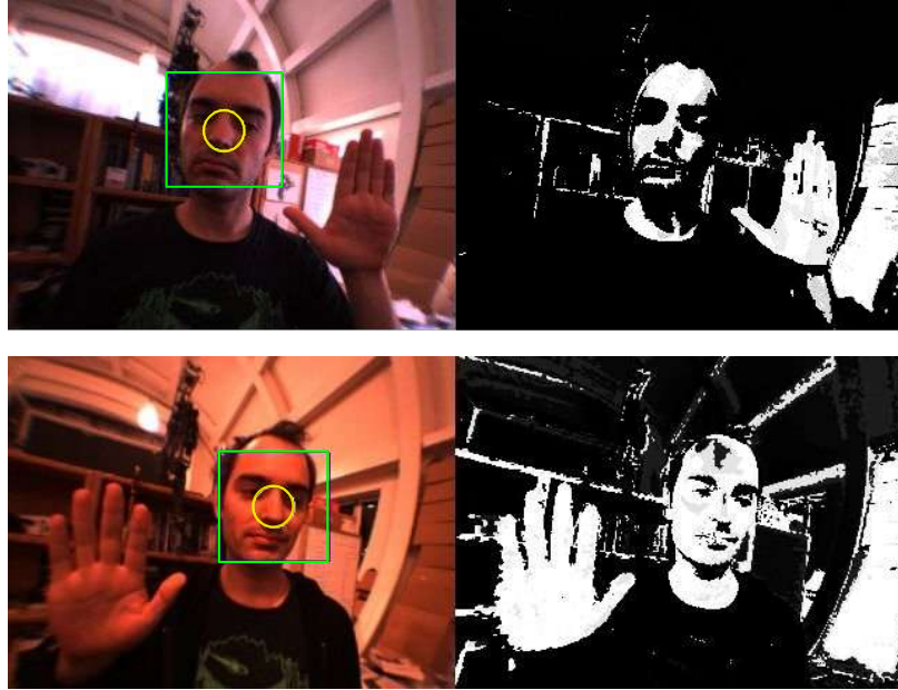
Figure 8-5: Output from the face tracker and skin color filter. The HSV skin color model adapts to the large shift in apparent skin hue between daylight (top) and night (bottom).
