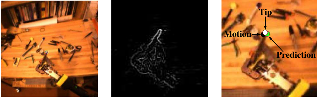
Figure 9-1: (Left) A typical view from the robot’s camera of the hand holding a pair of pliers. A naturally lit, cluttered background ensures a non-trivial environment for perception. (Middle) The tool tip is detected as the maximum point in the weighted edge map of the visual motor model. (Right) The raw motion-based detection (black), the hand-labeled tool tip (white), and a prediction based on the estimated tool position (green) are annotated.
