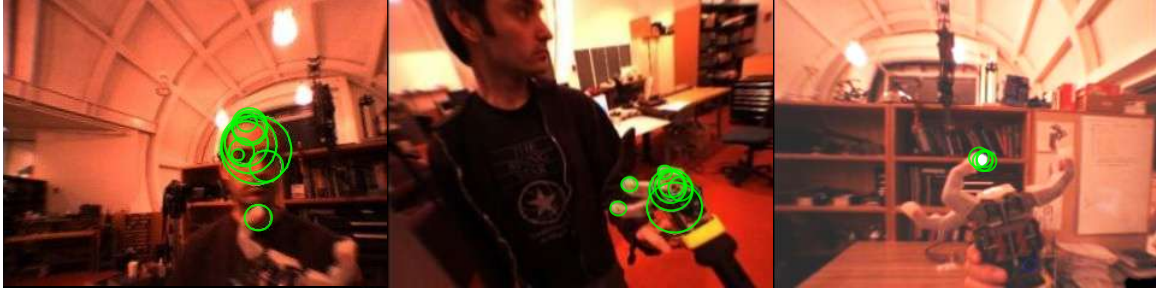
Figure 8-1: During human-robot interaction, faces, hands, and fingers, are important perceptual features for visual attention. As shown in green, the InterestRegions module will often select for these features because they are well modeled as rapidly moving convex edges.
