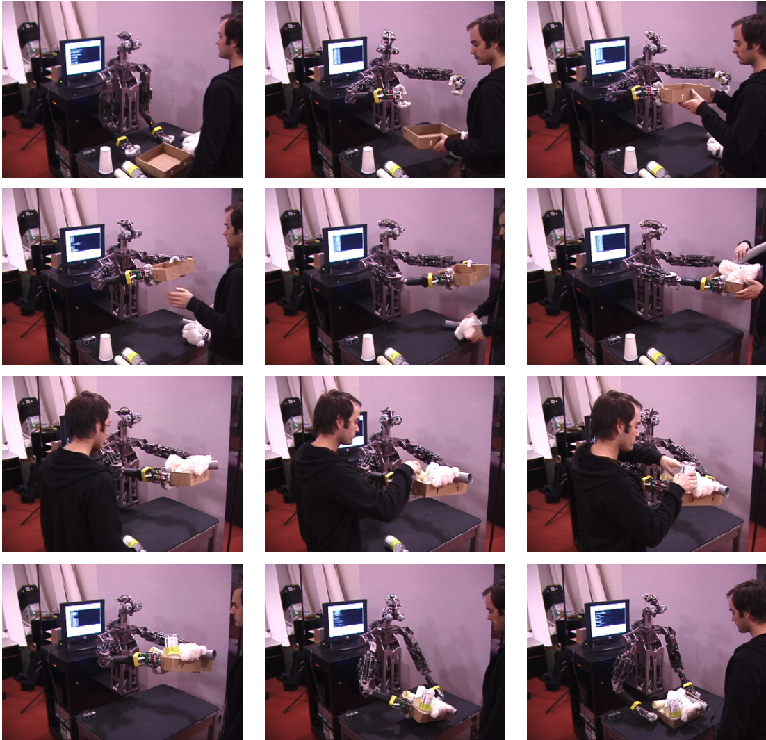
Figure 10-9: Domo assists a person in putting things away using the BimanualFixture module.
