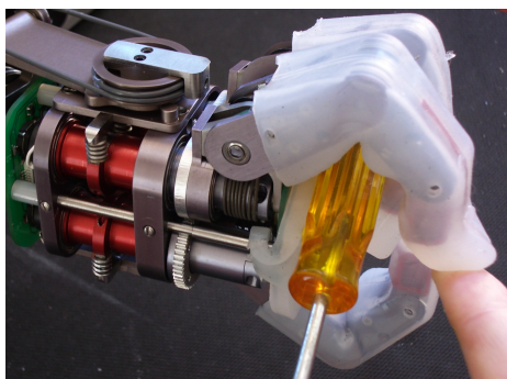
Figure 4-8: Domo's hand shown grasping a screwdriver (with a human finger for scale). The two 4 DOF hands that are approximately of human size and shape. Force sensing and control, combined with a compliant skin, allows them to maintain grasps on many everyday objects such as hand tools.
