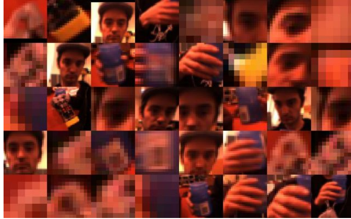
Figure 8-2: A random sample of image patches collected by the InterestRegions module. These predominantly contain hands, fingers, and faces. The lighter, grey colored patches correspond to the robot's hand.
