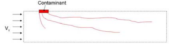
Fig. 8. Contaminant leak from a plant seeped through the ground and transported to other areas.
