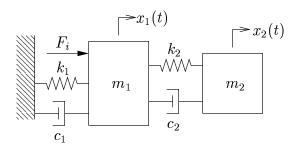
The voice coil exerts a force  $F_i$  on the bearing shaft  $m_1$ , and the LVDT produces a voltage  $v_1$  that is proportional to its displacement  $x_1$ .
