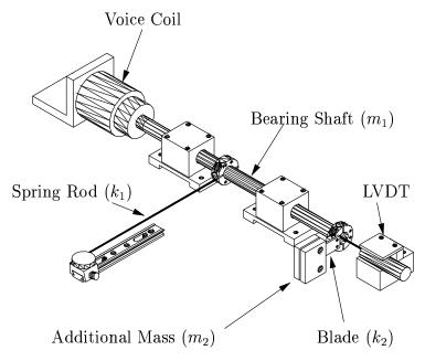
As in Lab 3, the bearing shaft (along with attached collars, LVDT core, voice coil, etc.) form a lumped mass  $(m_1)$ , the slender spring rod behaves as a massless spring  $(k_1)$ , and the voice coil serves as a force actuator as well as a damper  $(c_1)$ . The additional mass  $(m_2)$  is attached to this system via a thin aluminum blade that can be reasonably modeled as a massless spring  $(k_2)$  with light damping  $(c_2)$ . Therefore, our model of the system is:
