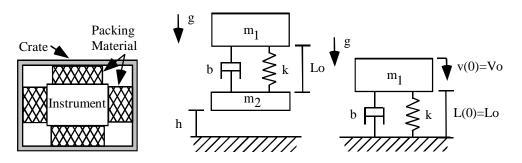
The packing crate (with instrument inside) is dropped from a height, h, as shown in the middle figure. The height is sufficiently large that by the time the crate hits the ground, the spring is fully extended to its unloaded length, Lo, as shown in the figure on the right. Note that the crate hits the ground with velocity,  $V_o$ , and in the presence of gravity.
