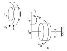
This problem ask us to collapse the gear train into the  $\omega_1$  frame. There are a number of methods to do this including doing force balances at each gear and using the the know relationships between the gear ratios to substitute for  $\omega_2$  and  $\omega_3$ . A simplier method would be to determine the equivelent interia and damping using the relationships in table 4.3-1 and collapse the system starting the in  $\omega_3$  frame. In the  $\omega_3$  frame:
