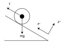
Using the analysis of pp. 17-19, we can calculate a dynamically equivalent mass for the wheel with its inertia:
