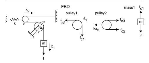
a) For part a, we are told that the mass and inertias of the pulleys are negligible thus summing the forces at each node results in the following:
