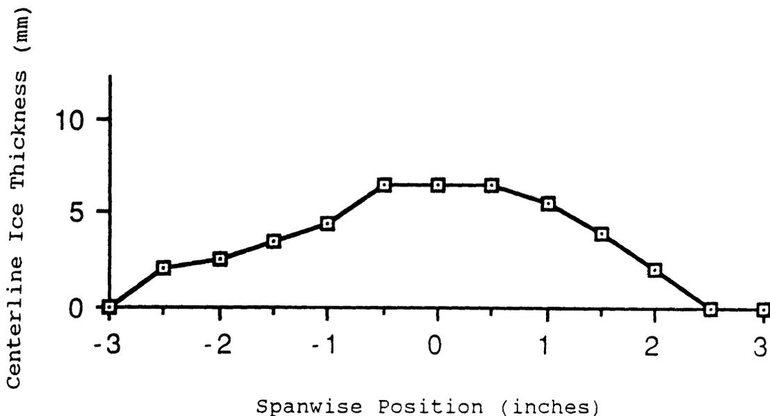
Figure 5-2 Centerline Spanwise Ice Thickness Variation Across Test Section
