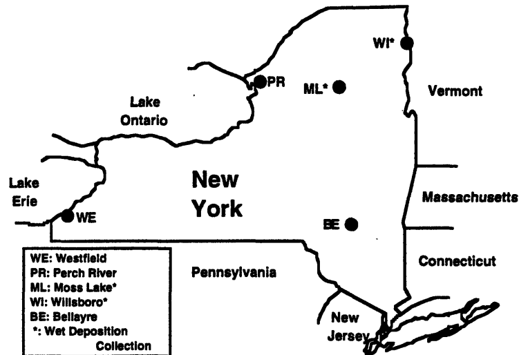
Figure 18. Atmospheric sampling locations in Upstate New York. Vapor-phase mercury and atmospheric particulates were collected at all five sites, and wet deposition was collected only at Moss Lake and Willsboro.
