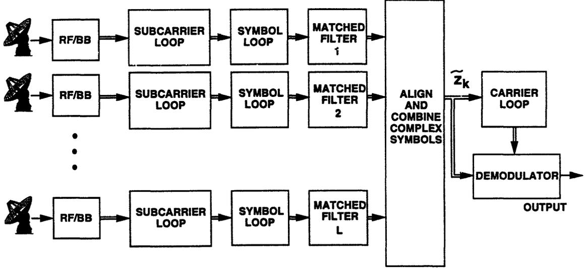
Figure 2-4: Block diagram of complex symbol combining
