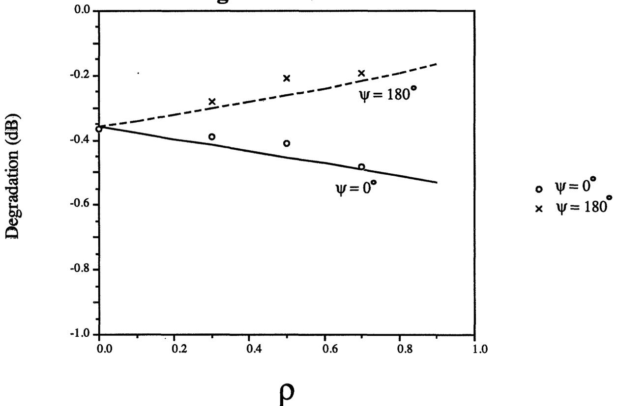
Figure 4-9: FSC degradation - theory and simulation
