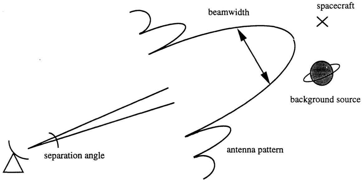
Figure 3-1: Spacecraft and background source in common beam
