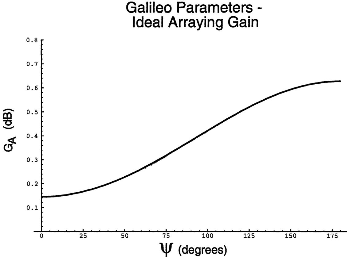
Figure 6-1: Ideal arraying gain for Galileo signal, array of DSS-14 and DSS-15
