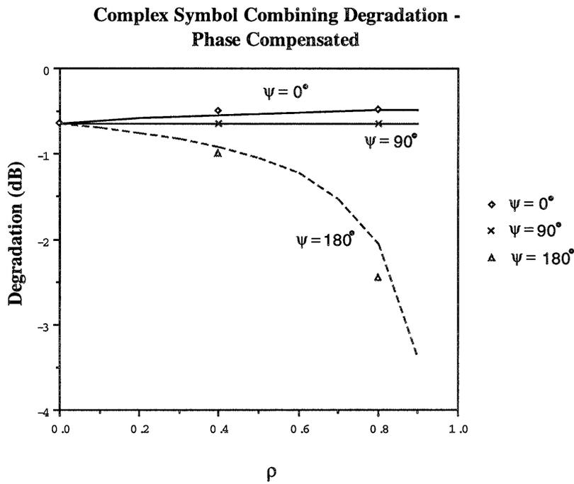
Figure 5-3: CSC degradation - theory and simulation
