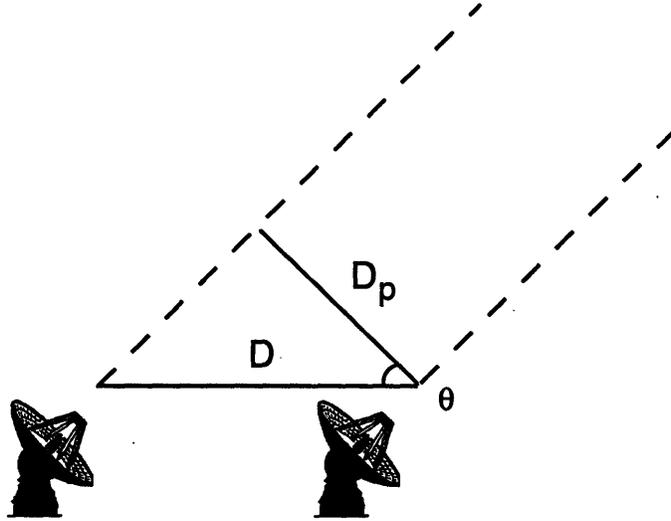
Figure 3-2: Antenna pair tracking distant source
