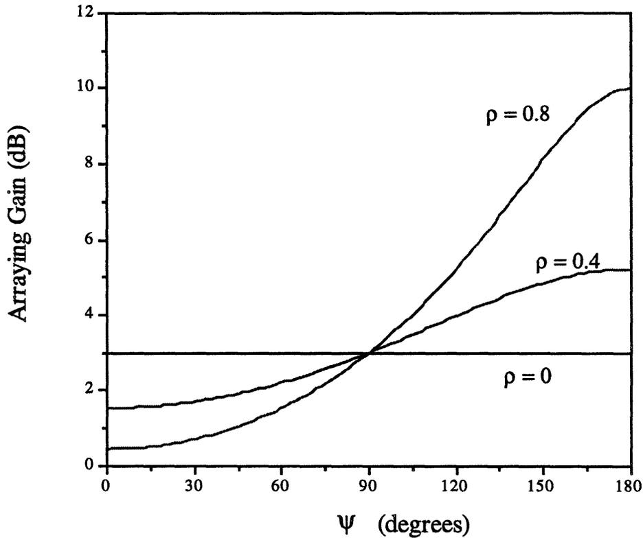
Figure 4-1: Ideal arraying gain  $G_A$  for various  $\rho, \psi$
