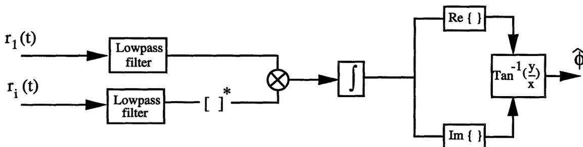
Figure 4-2: Conventional phase estimator
