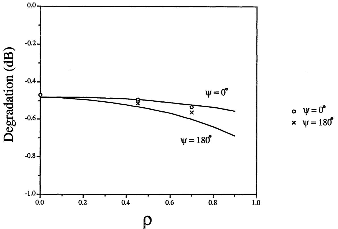
Figure 4-10: FSC degradation - theory and simulation
