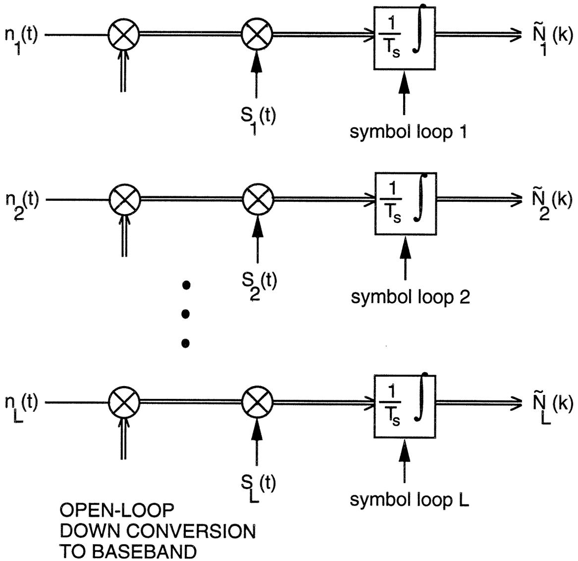
Figure 5-1: Matched filter noise outputs for CSC
