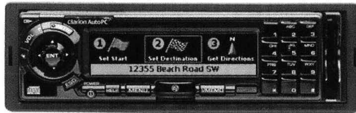
Figure 2.4: The Clarion AutoPC , a mobile communication, navigation and information system for automobiles. The faceplate provides buttons and controls for interaction, and a LCD screen with an icon based user-interface. Voice commands will allow hands-free control, along with text-to-speech for hearing status information.
