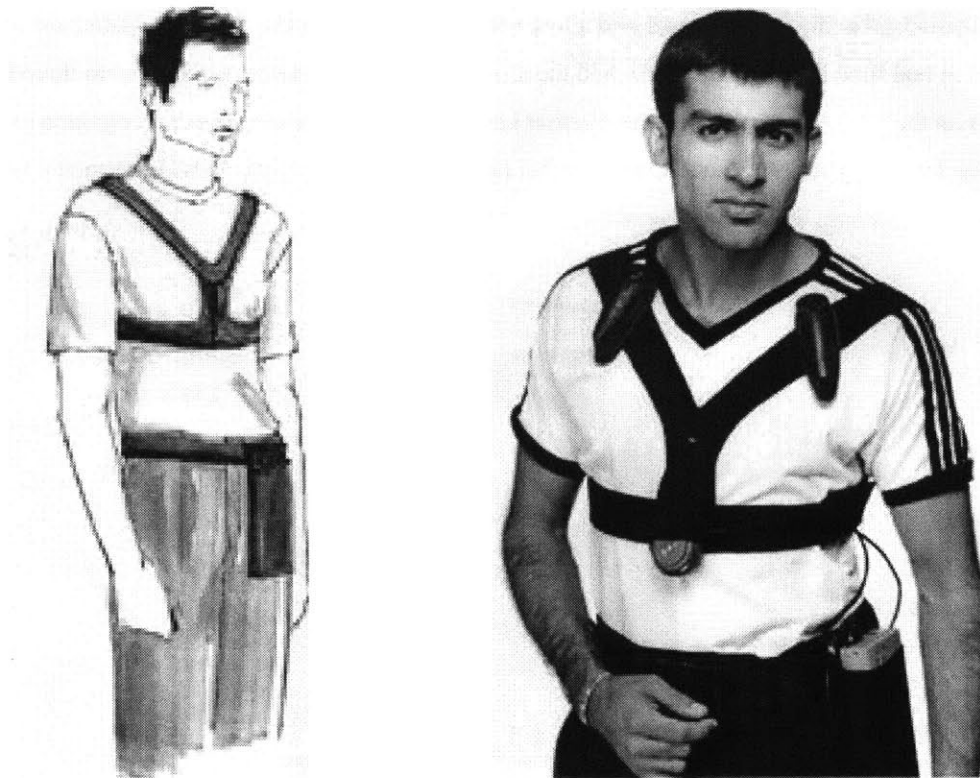
Figure 3.4: The Radio Vest , conceptual design and final implementation of an outdoor wearable configuration with clip-on directional speakers and powered microphone.
