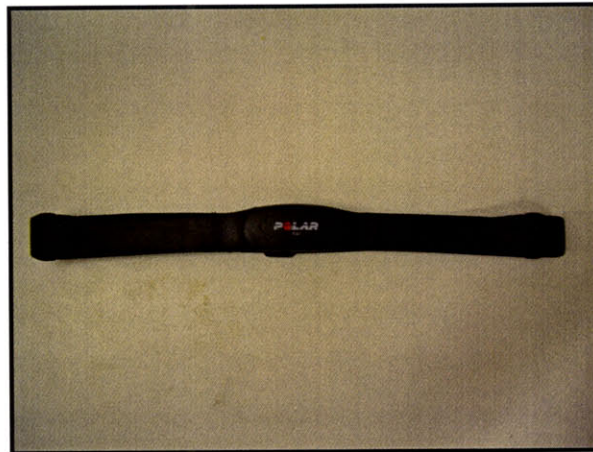
Figure 16: Non-invasive heart rate chest strap for detecting inter-beat interval of the heart. These types of sensors are very robust in the presence of large physical motion and have been shown to be highly correlated to more invasive ECG monitoring equipment. Most of the heart rate features of interest (such as heart rate variability measures) do not require ECG morphology information, so a non-invasive chest strap is just as ideal for heart rate sensing.
