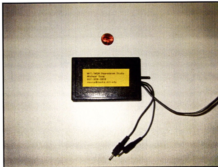
Figure 12: Bluetooth Location Beacon and associated housing and power supply. These beacons allow the LiveNet system to track the location of a patient within living spaces. The location beacons are completely adjustable in range, with an effective radius between ten and over several hundred ft.
