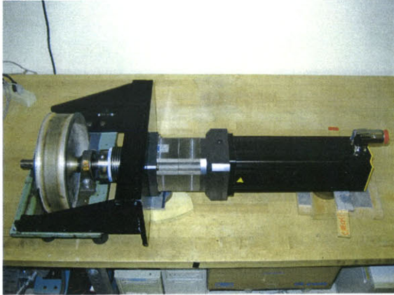
Figure 14. Motor/bracket/pulley configuration prior to final assembly.
