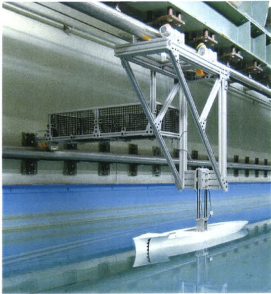
Figure 20. Front-quarter view of the light-weight carriage and Series 60 model.
