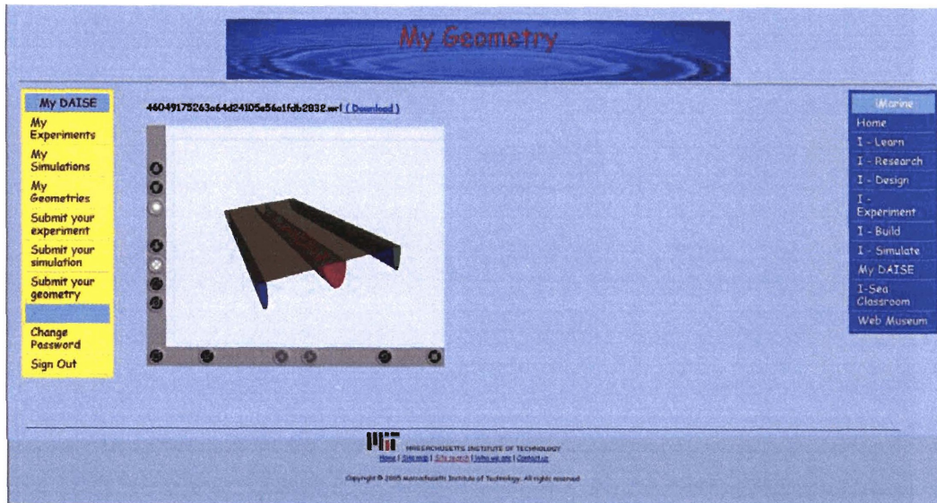
Figure 3-5: Geometry Graphic Interface. The user can have a 360 degrees view of the vessel created using the commands of the interface. The graphical interface is very useful for a quick check of the characteristics of the vessel under analysis.
