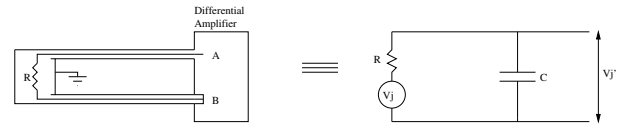
FIG. 1: Equivalent circuit of the thermal emf across a conductor of resistance R connected to a measuring device with cables having a capacitance C
