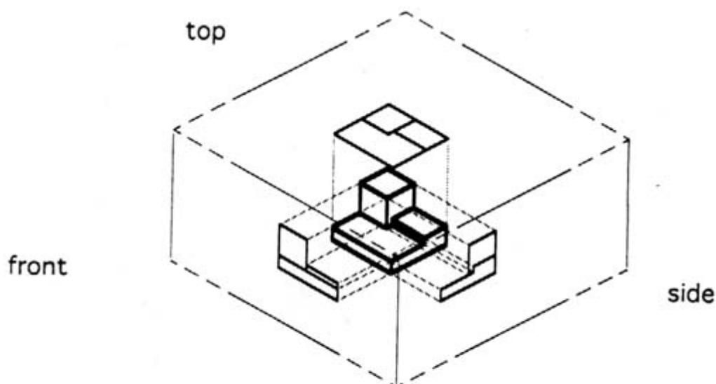
Figure 4 The block suspended in a glass box.
