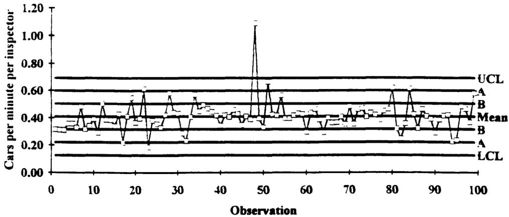
Figure 5-12: Control chart for the outbound inspection process.
