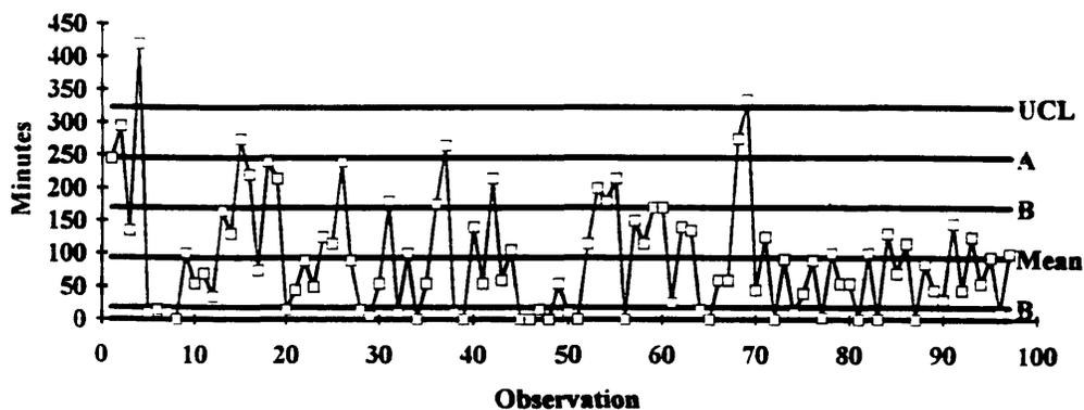
Figure 5-8: Control chart for those done assembling to start of inspection.
