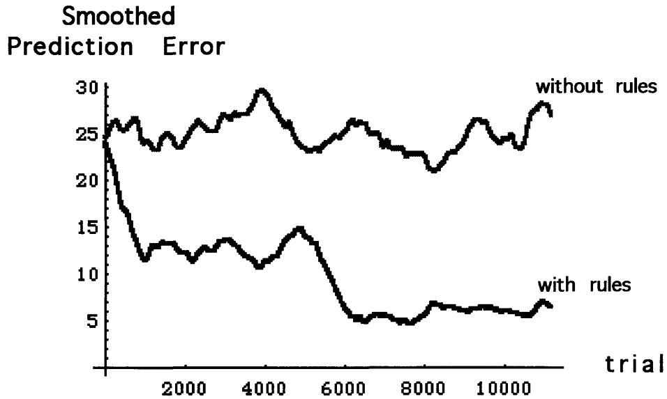
Figure 3-12: A graph of the smoothed error values as the agent learns the OV relation (the black line) compared with the smoothed error for an empty model (the gray line). To make this graph the prediction errors that the agent makes are further smoothed by averaging a window of 1000 trials. The agent is learning NOACTION rules only in the first 5000 trials.
