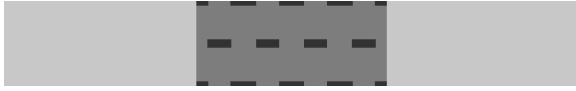
Fig. 9. Rectangles of aspect ratio 1:3 with short face normal to incidence radiation with larger dielectric constant embedded in a lower dielectric constant matrix.
