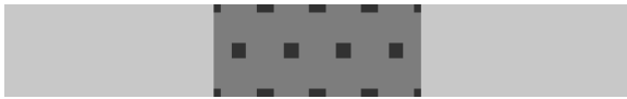
Fig. 7. Square nano-particles with larger dielectric constant embedded in a lower dielectric constant matrix.
