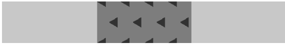
Fig. 10. Equilateral triangle nano-particles with vertex oriented towards incidence radiation with larger dielectric constant embedded in a lower dielectric constant matrix.
