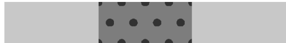
Fig. 6. Circular nano-particles with larger dielectric constant embedded in a lower dielectric constant matrix. The numerical effective medium results can be compared to an analytic result for this case.
