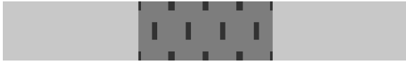
Fig. 8. Rectangles of aspect ratio 3:1 with long face normal to incidence radiation with larger dielectric constant embedded in a lower dielectric constant matrix.
