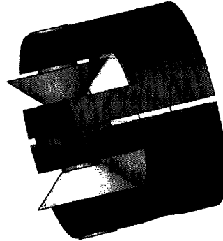
Figure 5: CAD model of final gearbox, showing gears meshed and dowel pins that hold the two perpendicular gears.
