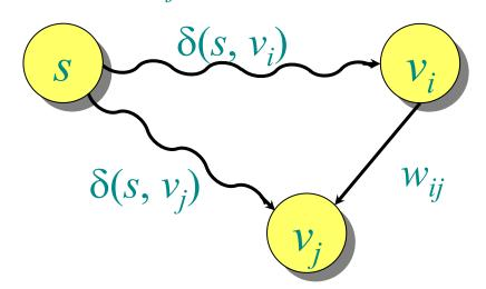
The triangle inequality gives us  $\delta(s, v_j) \le \delta(s, v_i) + w_{ij}$ . Since  $x_i = \delta(s, v_i)$  and  $x_j = \delta(s, v_j)$ , the constraint  $x_j - x_i \le w_{ij}$  is satisfied.
