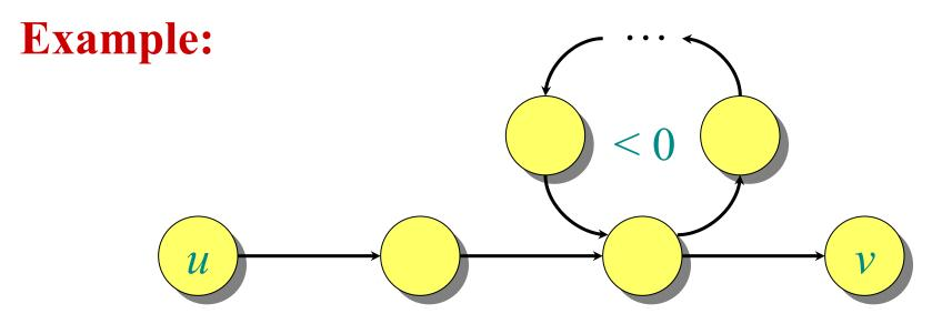
**Bellman-Ford algorithm:** Finds all shortest-path lengths from a **source**  $s \in V$  to all  $v \in V$  or determines that a negative-weight cycle exists.
