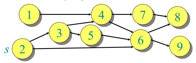
Walk through the vertices  $u \in V$  in this order, relaxing the edges in Adj[u], thereby obtaining the shortest paths from s in a total of O(V + E) time.
