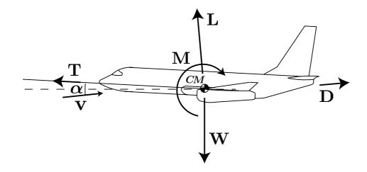
For steady level flight, the sum of the total forces and moments acting on the aircraft must vanish. It is clear that this must be the case, otherwise the aircraft would experience acceleration.
