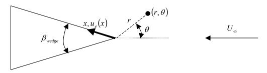
a) In order to estimate the behavior of the boundary layer on the wedge, the edge velocity is needed. Assuming the boundary layers are thin, we can estimate the edge velocity as the potential flow velocity on the body surface. The potential for wedge flow has the following form:
