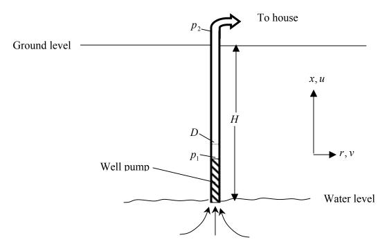
Assuming that the flow in the pipe is laminar and steady, derive the velocity distribution, u=u(r) that would exist in the pipe if the changes in the velocity are negligible in the xdirection. Start from the incompressible, steady, axisymmetric Navier-Stokes equations which are:
