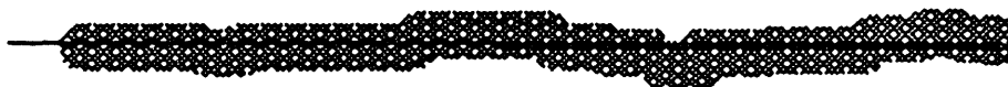
Short Tracks - Densely Ionized Interaction with Little Separation Associated with Alpha and High Energy Charged Particle Radiations
