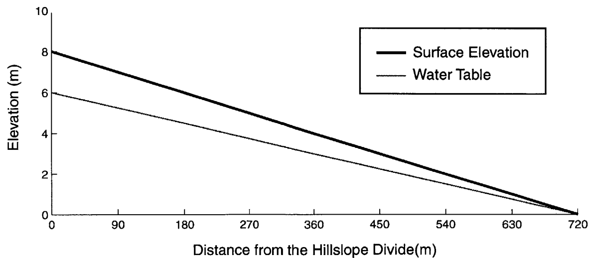
Figure 5-2: Cross-Sectional view of the hillslope used to test tRIBS
