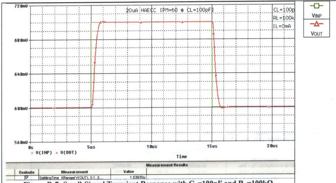
Figure D-7: Small-Signal Transient Response with C_L=100\text{pF} and R_L=100\text{k}\Omega
