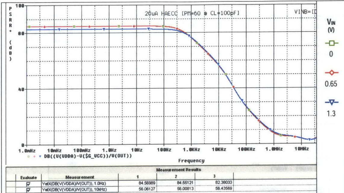
Figure D-5: PSRR+ vs Frequency with V_{IN}=0, 0.65, 1.3V
